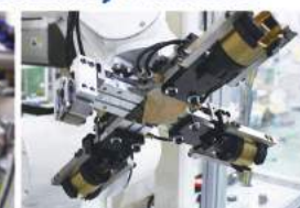
組入扣環 Circlip press fit by robot
