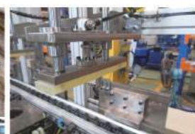
檢測三相電壓端子 Testing three-phase voltage terminal
