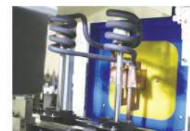
高週波機加熱鐵芯 High frequency heating lamination
