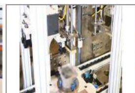
檢測扭力值 Inspect screw tighten torque
