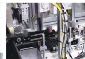
矽鋼片厚度檢測 Lamination thickness detection
